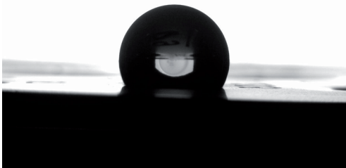
Fig. 4: The left image was taken with the room lights on and no collimating mask. The drop edge is not well-defined. The right image was taken in a dark room with the collimating mask on the light source. The drop edge is sharp and distinct
